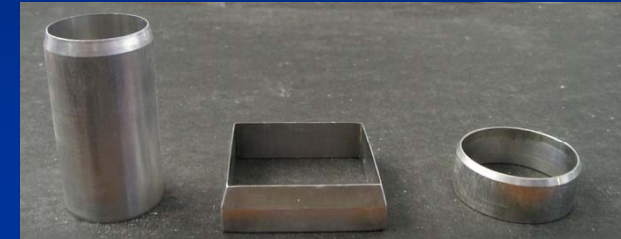
Preparation for Triax, shear, edo. (steel)
